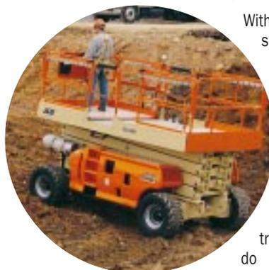
With a new twin pump power 4WD system, the RT Series provides a higher level of performance over rough terrain. Each pump provides full power to all wheels without the inefficiencies common on competitive machines. "Superwide" tyres provide outstanding flotation while a standard oscillating axle allows for optimum wheel contact and greater traction. Plus, the four-wheel brakes do what competitor's dual brakes can't—hold on the same grades.
