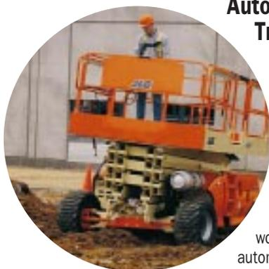
In order to help you work efficiently, JLG left nothing on the RT Series to chance. A manual speed selector allows you to choose between low, medium and high speeds to match your specific working conditions. Plus, an automatic transmission provides the power when travelling up a grade and helps control the descent when going down a grade.
